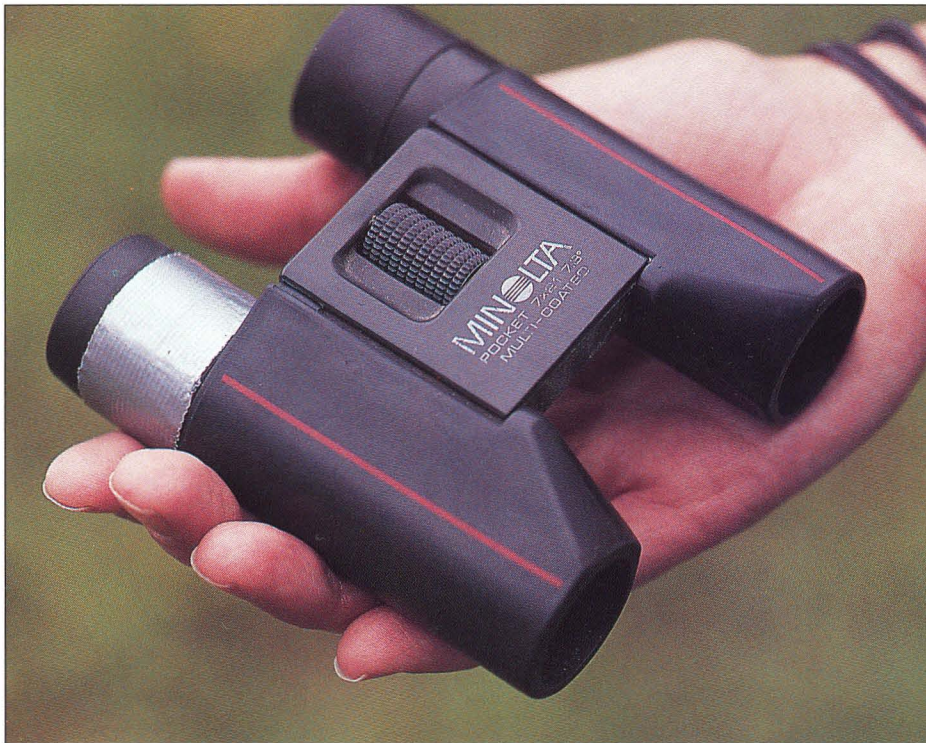
The diopter adjustment allows for differences in the viewer's eyes. It's a good idea to tape the setting in place to avoid adjustment every time you look.
