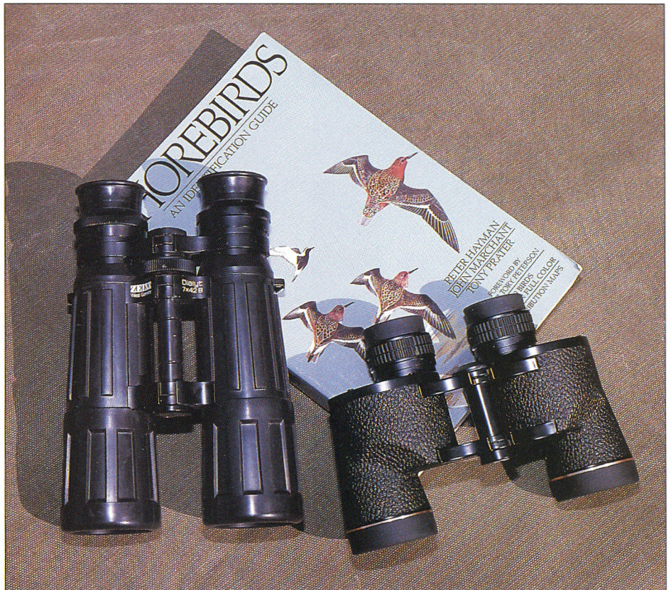
Two general types of binoculars are built; the roof prism, left, and the porro prism, right. Good roof prisms are lighter and compact but more expensive.
